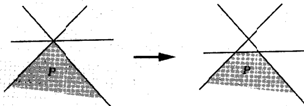
Figure 2.10: Small changes in the constraining inequalities can remove degeneracy.
