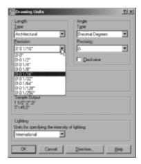
FIGURE 3.3: The Precision drop-down list for architectural units
