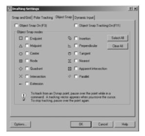
FIGURE 4.30: The Object Snap tab of the Drafting Settings dialog box
