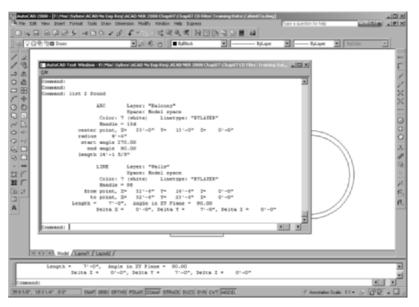
FIGURE 7.13: Toggling between the Text Window (above) and the drawing with its Command window (next page)
