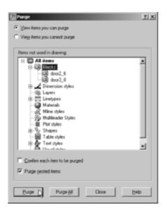
FIGURE 9.27: Deleting the block references with the Purge dialog box
