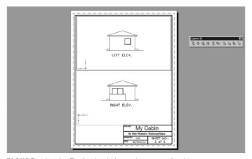
FIGURE 14.18: The elevations in the two viewports are aligned.
