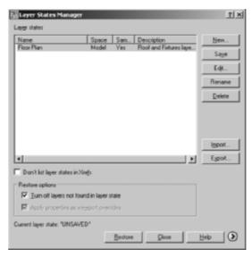
FIGURE 6.37: The Layer States Manager dialog box showing the new layer state
