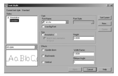
FIGURE 8.2: The Text Style dialog box, in which text styles are set up
