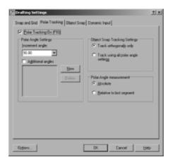
FIGURE 6.32: The Polar Tracking tab in the Drafting Settings dialog box
