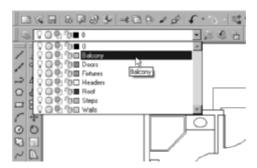
FIGURE 6.14: The opened Layer Control drop-down list
