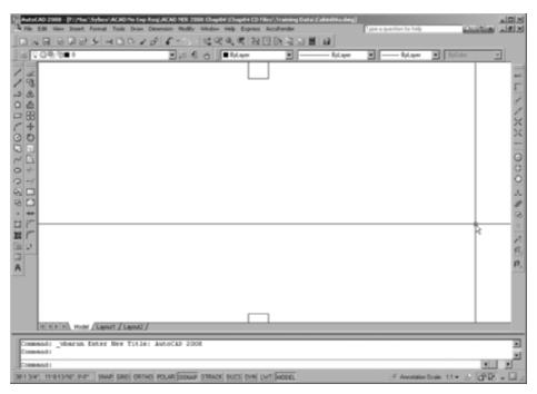
FIGURE 4.43: The Object Snap toolbar docked to the right of the drawing area
