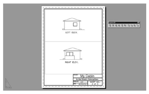
FIGURE 14.15: The Cabin RElev layout after rotating the UCSs and adjusting the view-ports' content
