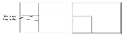
FIGURE 4.12: Selecting the second two lines to fillet (left) and the result of the second fillet (right)
