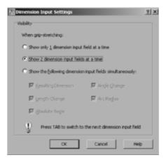
FIGURE 3.17: The Dimension Input Settings dialog box
