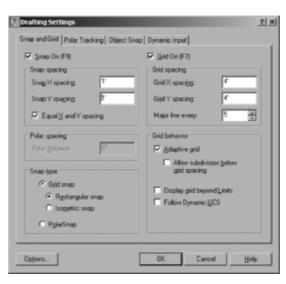
**FIGURE 3.9:** New settings on the Snap and Grid tab of the Drafting Settings dialog box
