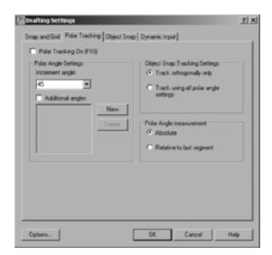
FIGURE 5.4: The Polar Tracking tab of the Drafting Settings dialog box
