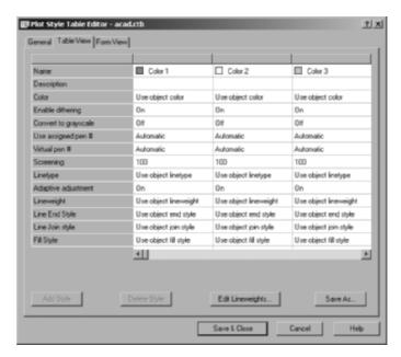
FIGURE 15.20: The Table View tab of the Plot Style Table Editor dialog box for the acad.ctb file
