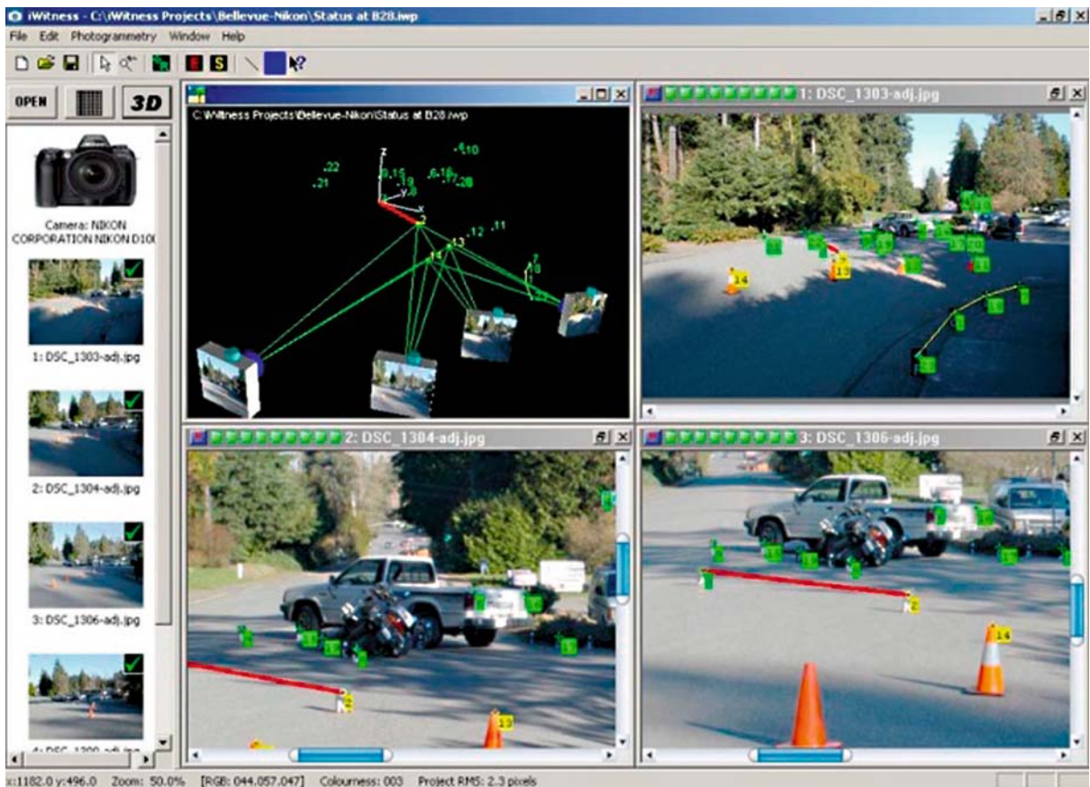
Photogrammetric Applications, Figure 6 Accident scene recording and photogrammetric processing (Photomatrix)
