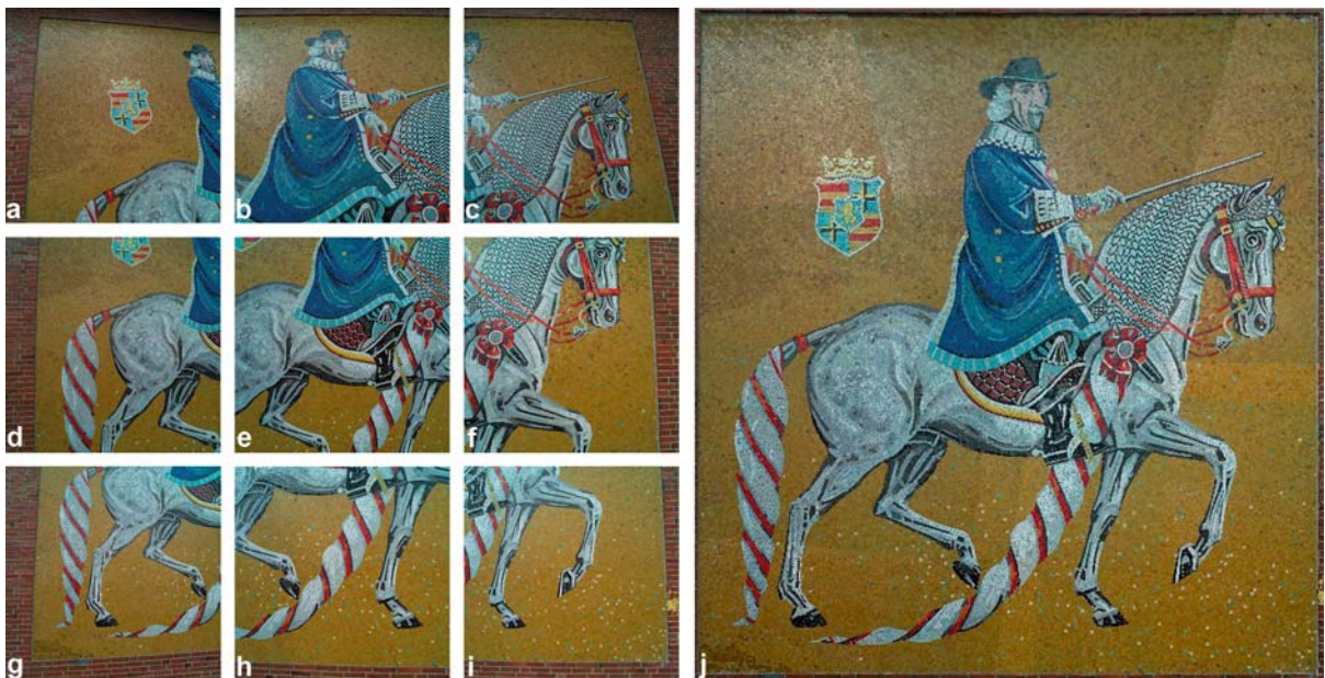
Photogrammetric Applications, Figure 4 Original images (a–i) and resulting orthophoto mosaic (j)(IAPG Oldenburg)
