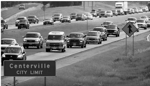
Contraflow in Transportation Network, Figure 2 Hurricane Rita evacuation required contraflow on Interstate Highway 45. Notice that traffic on both sides of I-45 is going north (source: dallasnews.com)
