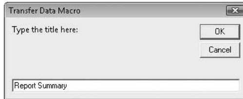
Figure 3-4 An input box is a simple dialog box that contains a single text field and OK and Cancel buttons.
