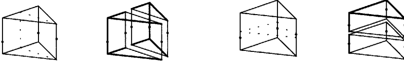
Figure 23.6. Split of a \times -simplex and new positions of the barycenters \xi_{v_i} .
