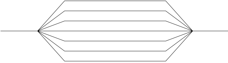
Fig. 2. Schematic representation of a double ended hump yard. The hump is present on just one of the two tracks connecting to the classification tracks (e.g., on the right hand side).
