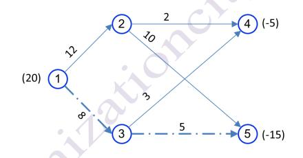
In the above figure, arcs \_\_\_\_ indicate non-basic arcs that are at their upper bound, and arcs \_\_\_\_ (solid arcs) are basic arcs. Solid arcs form a spanning tree for the network, which is the basic solution. To determine whether the current solution is an optimal basic solution, the cost  $\overline{c_{ij}}$  of all non-basic arcs must be calculated. For this purpose, we first calculate y<sub>i</sub> (i=1,2,...,n). If the y<sub>i</sub> applies in the following relations:
