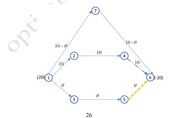
The arc (1,7) leaves the base. Therefore, the current basic solution is as follows and the value of the objective is equal to 0.
