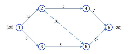
In this solution, the value of the objective function is equal to 155. According to the assumption  $y_2=0$ , the value of  $y_i$  can be calculated from the equations  $c_{ij}-y_i+y_j=0$  for the basic arcs as follows.
