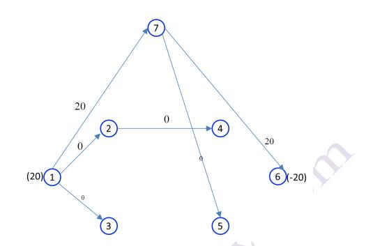
In this iteration, the value of the objective function is equal to 40. Assuming  $y_7=0$ , the y<sub>i</sub>s can be obtained based on  $c_{ij}-y_i+y_j=0$ .
