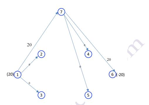
In this iteration, the value of the objective function is equal to 40. Assuming  $y_7=0$ , the y<sub>i</sub>s can be obtained based on  $c_{ij}-y_i+y_j=0$ .
