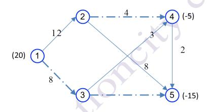
According to the assumption  $y_2=0$ , the value of  $y_i$  can be calculated from the equations  $c_{ij}-y_i+y_j=0$  for the basic variables as follows.
