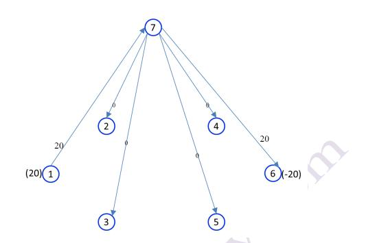
Assuming  $y_7=0$ , the  $y_i$  coefficients can be obtained based on  $c_{ij}-y_i+y_j=0$ .
