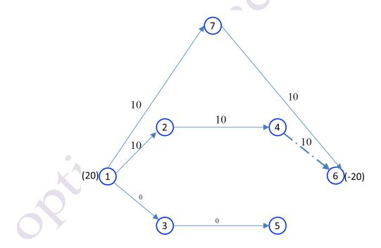
Assuming  $y_7=0$ , the  $y_is$  can be obtained based on  $c_{ij}-y_i+y_j=0$ .
