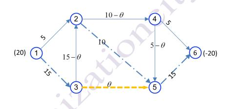
With  $\theta$ =5, the arc (4,5) leaves the base and the arc (3,5) enters the base. With this change, the current solution is as follows.
