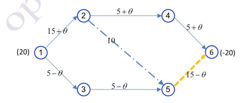
With  $\theta$ =0, the arc (1,2) leaves the base. Therefore, the current solution is as follows.
