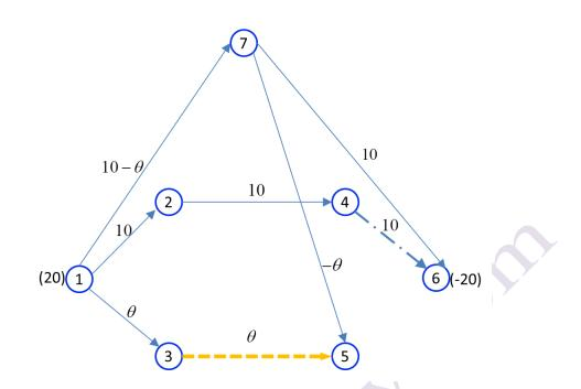
The arc (7,5) leaves the base. Therefore, the current basic solution is as follows and the value of the objective is equal to 20.
