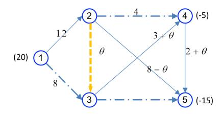
The value of  $\theta$  can be increased up to 8, in which case the arc (2,5) is removed from the basic solution, and therefore the basic solution is as follows.
