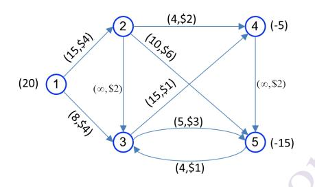
In the figure, there is (A, B) on each arc, where A represents the capacity of the arc and B represents the cost of passing one unit through the arc. Consider the initial solution below.
