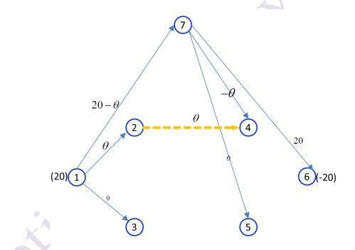
The arc (7,4) leaves the base. Therefore, the current basic solution is as follows.
