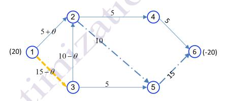
With  $\theta$ =10, the arc (3,2) leaves the base and the arc (1,3) enters the base. Therefore, the current solution is as follows.
