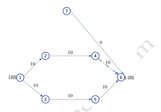
Assuming  $y_7=0$ , the  $y_is$  can be obtained based on  $c_{ij}-y_i+y_j=0$ .
