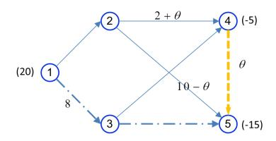
The value of  $\theta$  can be increased up to 2, in which case the arc (2,4) reaches its upper bound and leaves the basic solution. Therefore, the current basic solution is as follows:
