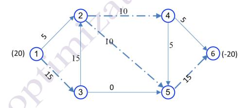
In this solution, the value of the objective function is equal to 295. According to the assumption  $y_2=0$ , the value of  $y_i$  can be calculated from the equations  $c_{ij}-y_i+y_j=0$  for the basic arcs as follows.
